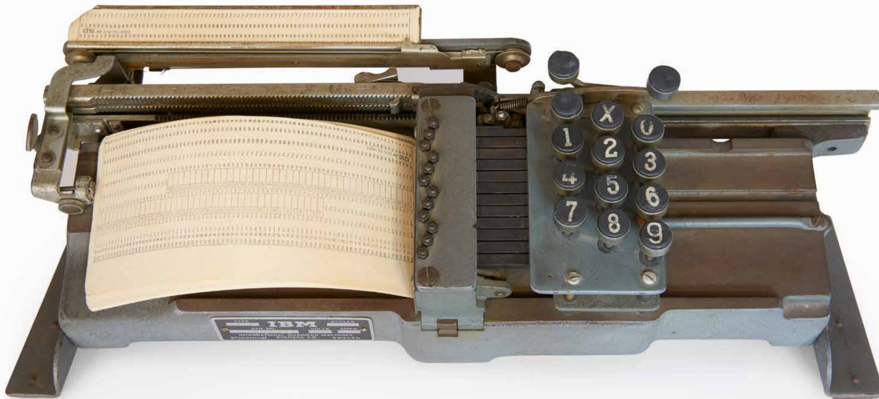
BEIJER'S FIRST 'COMPUTER', A PUNCHED CARD MACHINE FROM THE END OF THE 1940S, SUPPLIED BY THE SWEDISH BRANCH OF IBM. THE USE OF SUCH MACHINES TO STORE DATA REACHED ITS PEAK IN 1969 BUT THEY WERE GRADUALLY REPLACED BY WORKSTATIONS WITH SCREENS.
