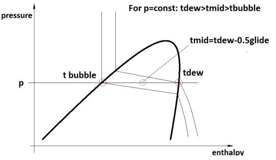
• If your controller receives set point as temperature, and works e.g. based on dew curve, remember to increase all set point by half of a glide for give pressure / pressure range:
