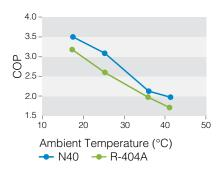
Emerson Climate Technologies also tested Solstice N40 in their Supermarket Laboratory and demonstrated up to 8% lower energy consumption in medium temperature and 3% in Low temperature regulated testing against R-404A.
