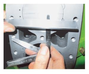
State of the art reassembly: Performance must be preserved, here checking the dead volume.
